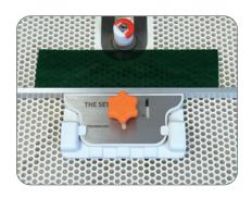
**4.** Place glass flush against the aluminum bar. Slide the Adjustable Plate until the glass makes contact with grinding bit.
