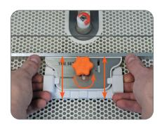
3. Loosen the Adjustment Knob counter clockwise and slide the Adjustable Plate to desired location.
