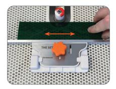
**6.** Place glass flush against aluminum bar and grind glass from **right** to **left**.
