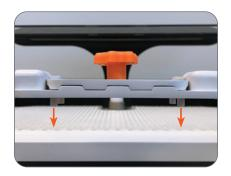
Turn off Grinder. Center THE SET horizontally across the Lift Grid, aligned with the grinding bit.
